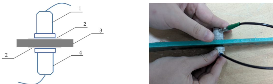
Figure 1. Shadow method of ultrasonic flaw detection (1—transmitting piezoelectric transducer; 2—glycerin layer; 3—experimental plastic sample; 4—receiving piezoelectric transducer).
