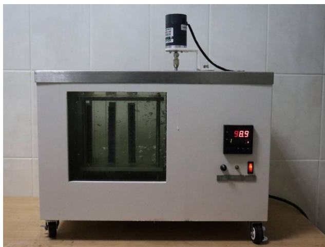
Figure 5. Photographs of several composite formulations during ESCR testing.
