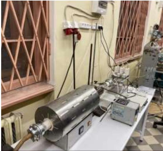
*Figure 2.2. Laboratory installation of CVD for obtaining ZnS*
